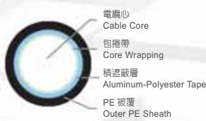
1 Conductor : Solid annealed copper wire size 0.4, 0.5, 0.63mm.
