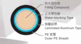
1 Conductor : Solid annealed copper wire in size 0.4mm to 0.65mm.
